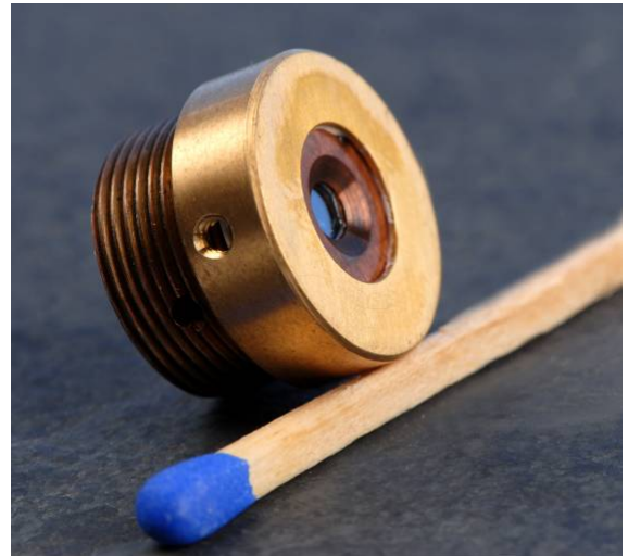
Fig. 1: OPSDL semiconductor structure with transparent heatspreader, mounted inside the VERTIGO submount. This mounted chip is the core for all different laser modules.
